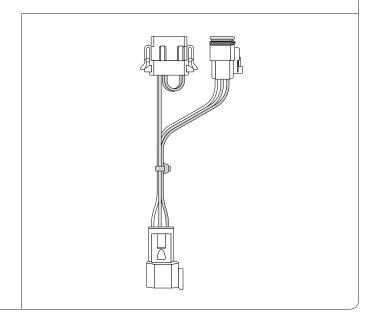
**3)** Connect the C1 connector into the G0 RUGGED device, and then mount the G0 RUGGED device in the best suitable spot according to the wire length and positioning for network and GPS connectivity.
